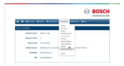
Select the button 'Check for update'. The BOSCH Coach MediaRouter loads and installs the latest available software. The download times depend on the mobile connection. All LEDs light up red.
